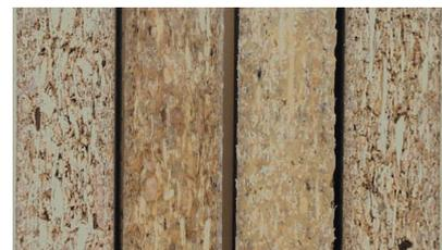
**Jowatherm-Hot Melt “filled” and “unfilled”:** Can you see the difference at 170 micrometer thick adhesive coating?
